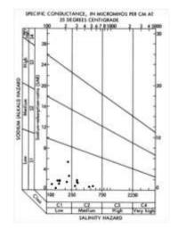
Figure (13) Sodium Adsorption Ration (SAR)
